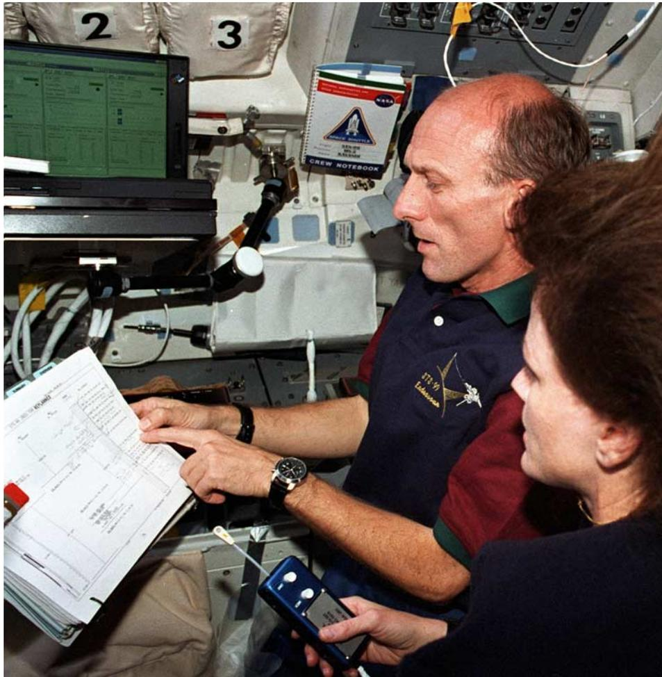
**Figure 9.** Mission Specialists Gerhard Thiele and Janet Kavandi go over the crew timeline in the shuttle aft flight deck. The laptop at top left is the recorder interface controller; its screen shows the status of three payload high-rate recorders (PHRR). Behind Thiele's arm are two PHRRs. Johnson Space Center photograph sts099\_327\_003.
